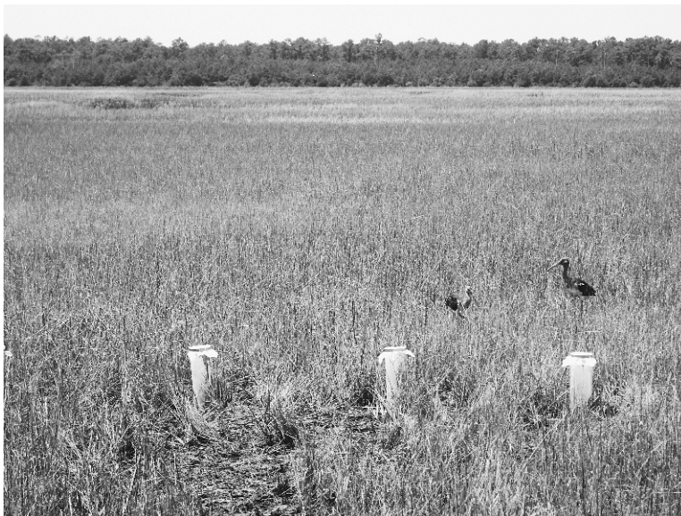
PLATE 1. To manipulate consumer access to Spartina alterniflora , we used cages made of four-inch (1 inch = 2.54 cm) PVC and mesh windows. The cages shown here are from the induction phase at site 3 in South Carolina, USA. Photo credit: J. D. Long.
